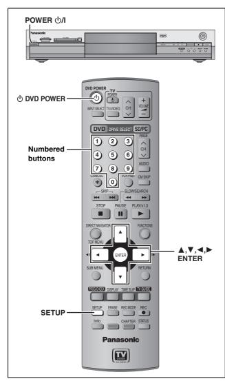
After plugging the unit into your household AC outlet and pressing [⊕ DVD POWER] to turn the unit on for the first time, the unit starts TV Guide On Screen™ system setup.
